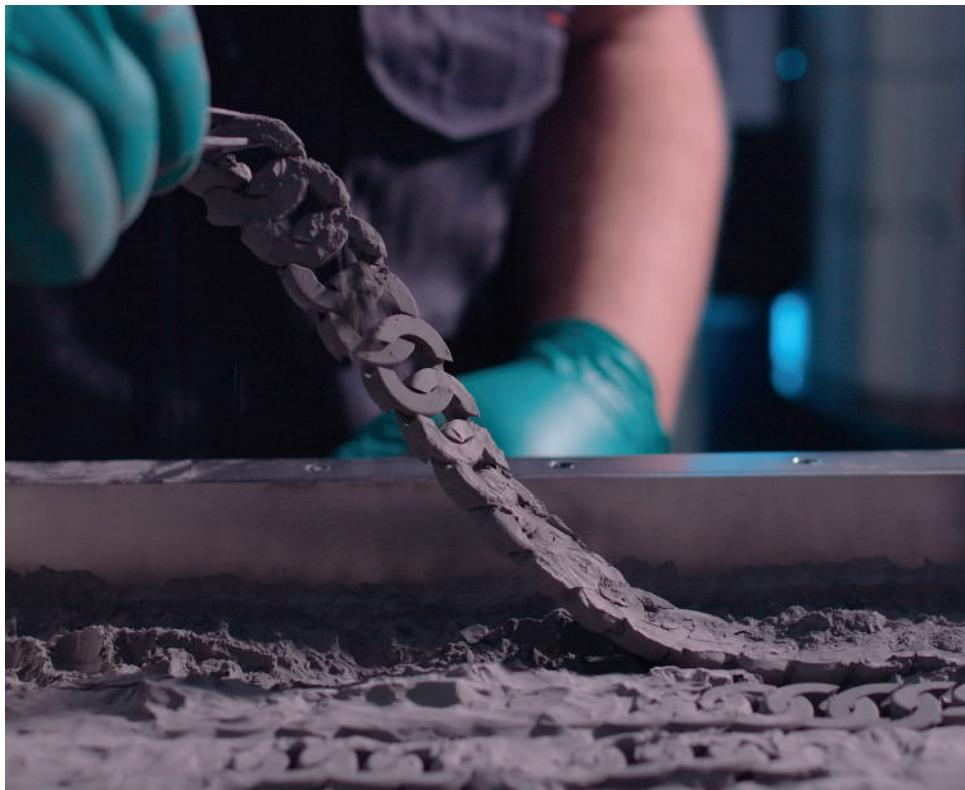
Binder Jetting is a **powder-bed 3D printing** technology offering unprecedented design freedom. This innovative process revolutionizes traditional manufacturing by shortening the supply chain and reducing development time. By eliminating the need for molds and tooling, it allows for greater production agility and a more sustainable approach.
