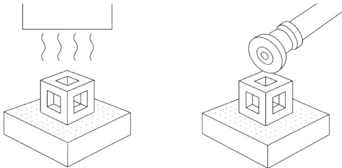
The part is heated to a temperature below the metal's melting point. The binder burns out, particles bond, and the piece densifies with up to 20% shrinkage.
