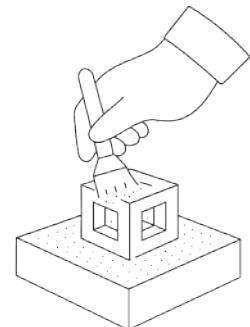
An inkjet printhead selectively deposits a liquid binder, layer by layer, onto a metal powder bed, creating the so-called "green part".
